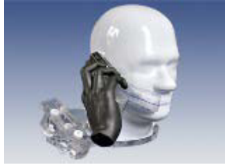
Figure 4.3 Example of a head phantom for SAR measurements 6
