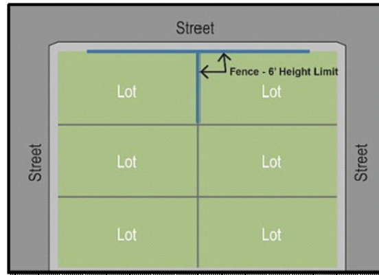
Figure 1120.04.1: 6-Foot Fence Height Limit
