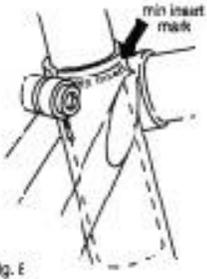
**circumstances should the seat post project from the frame beyond its "Minimum Insertion" or "Maximum Extension" mark (Fig. 8).**
