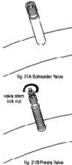
the valve cap and push the air hose or pump fitting onto the end of the valve stem. To let air out of a Schraeder valve, depress the pin in the end of the valve stem with the end of a key or other appropriate object.
